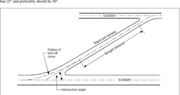
3.9.18 The intersection angle of a rapid exit taxiway with the runway shall not be greater than  $45^{\circ}$  nor less than  $25^{\circ}$  and preferably should be  $30^{\circ}$ .
