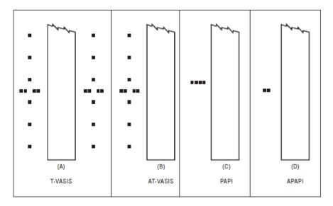
Figure 5-16. Visual approach slope indicator systems
