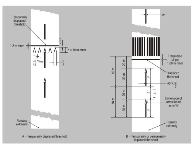
Figure 5-4. Displaced threshold markings
