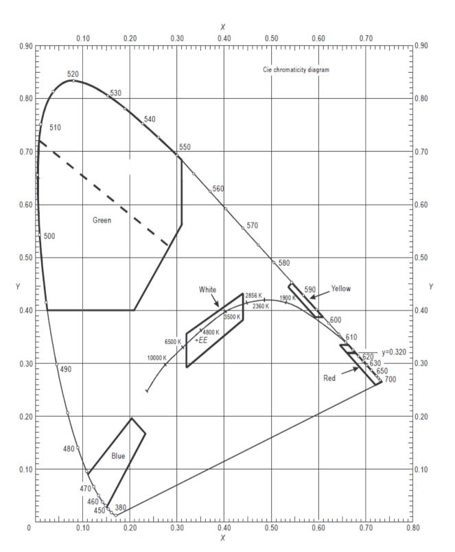
Figure A1-1b. Colours for aeronautical ground lights (solid state lighting)
