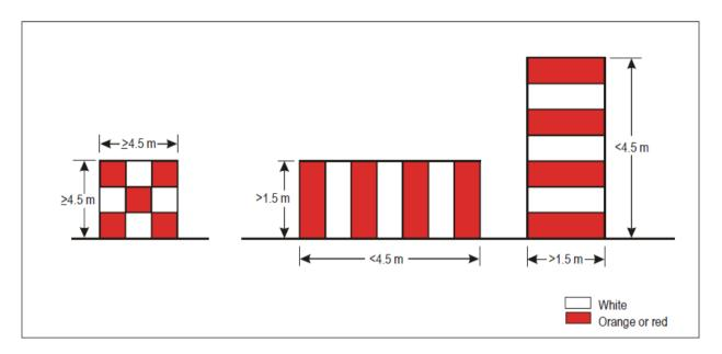
Figure 6-1. Basic marking patterns
