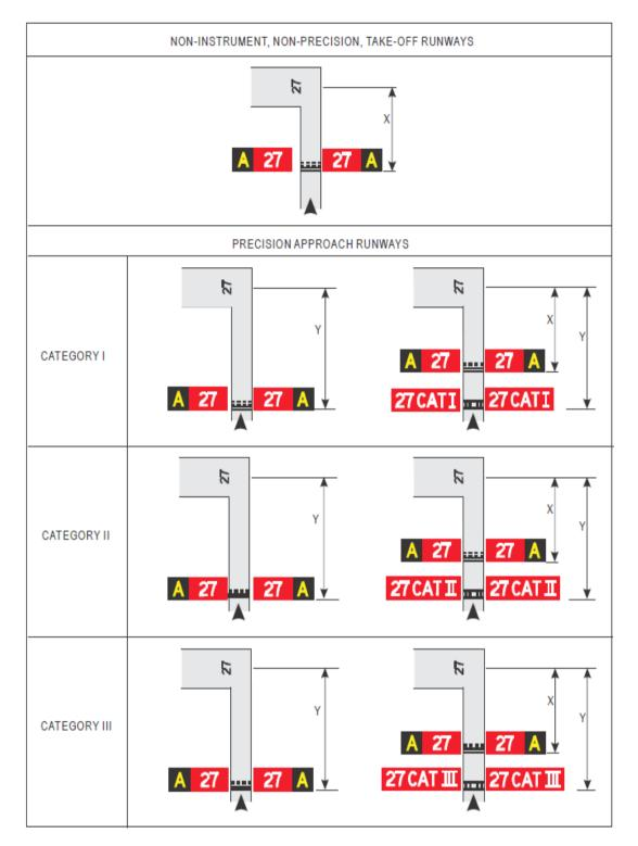
Note.— Distance X is established in accordance with Table 3-2. Distance Y is established at the edge of the ILS/MLS critical/sensitive area.
