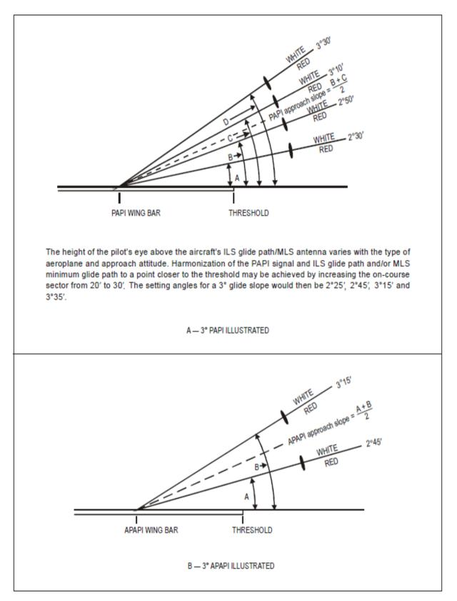
Figure 5-20. Light beams and angle of elevation setting of PAPI and APAPI
