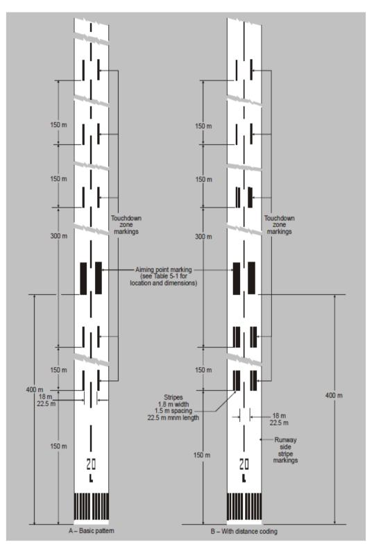
Figure 5-5. Aiming point and touchdown zone markings (illustrated for a runway with a length of 2 400 m or more)
