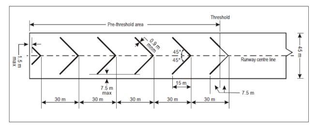
Figure 7-2. Pre-threshold marking
