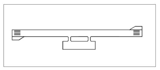
Figure 3-1. Typical turn pad layout
